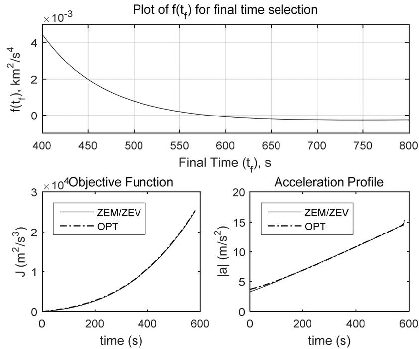
**Figure 4: Plots of  $f(t_f)$ , objective function, and acceleration for Case B**
