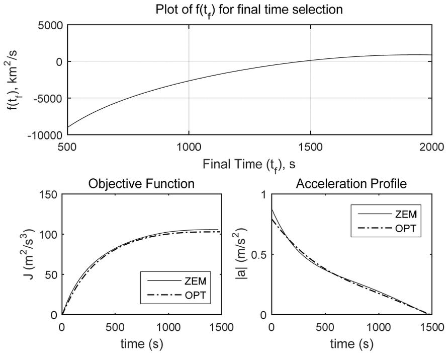
Figure 6: Plots of  $f(t_f)$ , objective function, and acceleration for Case C
