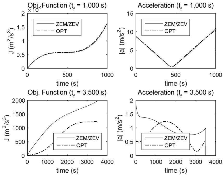
Figure 10: Objective Function and Control Input ( $t_f = 1,000 / 3,500$  sec.)
