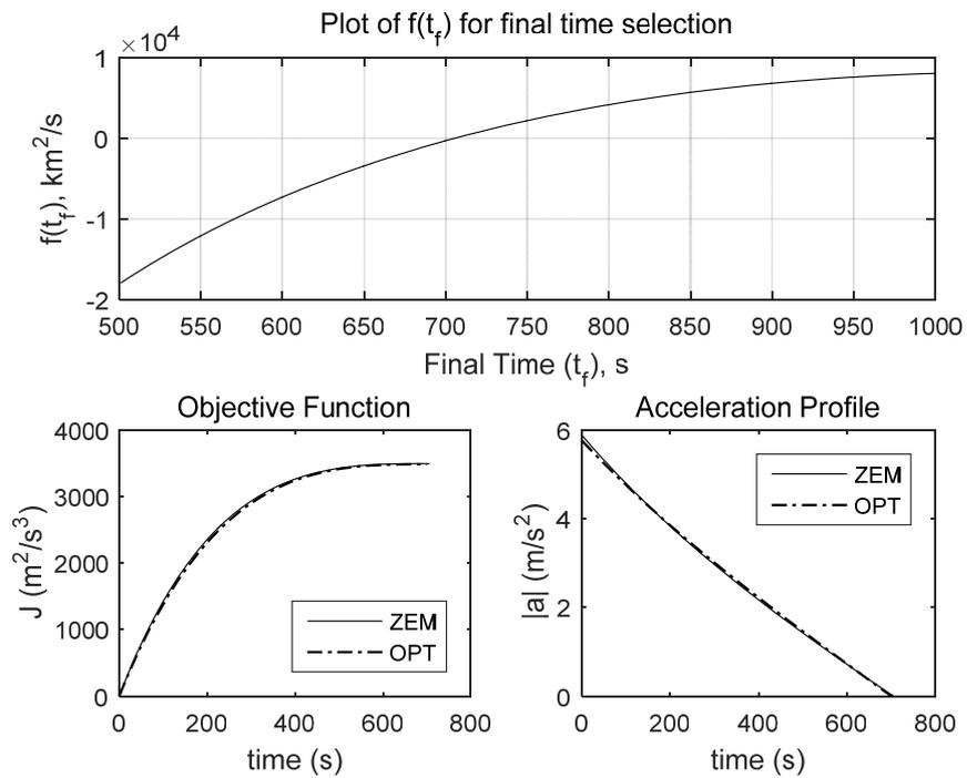
Figure 2: Plots of  $f(t_f)$ , objective function, and acceleration for Case A
