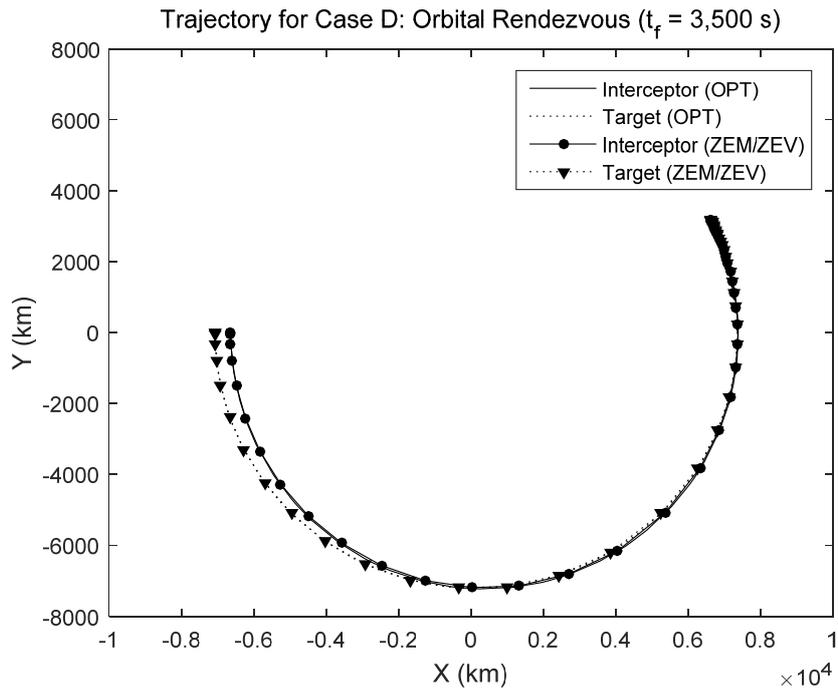
Figure 9: Trajectory for Case D – orbital rendezvous ( $t_f = 3,500$  sec.)
