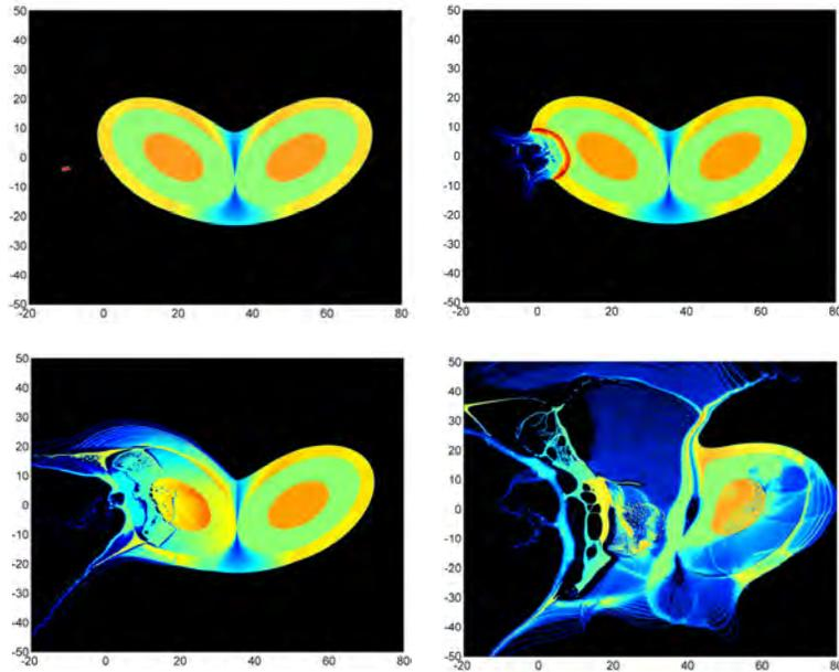
**Figure 2. A 70-m asymmetric 2D model disrupted by a 10-km/s kinetic-energy impact and a subsequent 70-kt nuclear subsurface explosion of the HAIV system [10–12].**
