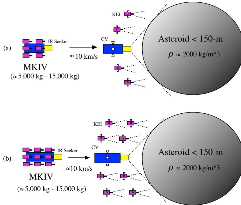
**Figure 3. Conceptual 2D illustration of a non-nuclear MKIV mission concept for dispersive pulverization of a small asteroid.**
