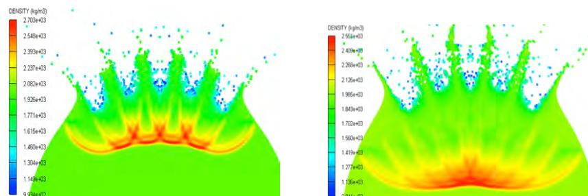
**Figure 12. Case 4 results for an ANSYS AUTODYN 2D model with Tillotson EOS.**
