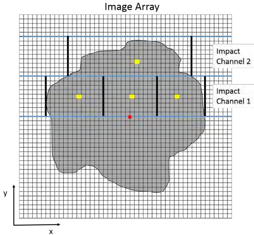
Figure 14. Graphical illustration of a multi-target terminal guidance algorithm for a reference MKIV system consisting of a CV and four KEIs.
