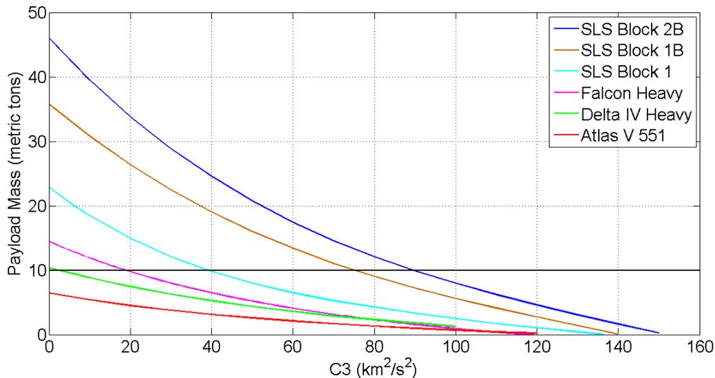
**Figure 16. Interplanetary mission capabilities of heavy-lift launch vehicles (Delta IV Heavy, Falcon Heavy and the SLS) compared to Atlas V 551 [29].**
